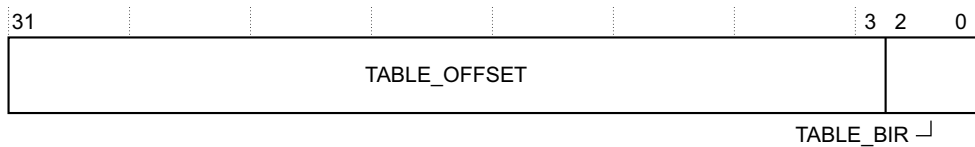
Figure 3-86 PCIE_PCI_IRQ_1 Register bit assignments
