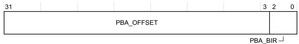
Figure 3-87 PCIE_PCI_IRQ_2 Register bit assignments
